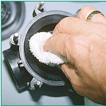
• **Diaphragm-style valves** – remove the bonnet, solenoid and diaphragm assembly; drain or sponge any standing water; then reassemble. Leave the solenoid in open position for winter.
